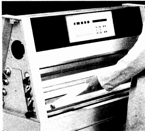
QUV/se does not require lamp rotation. However, when the time comes to change a lamp, double sided access makes the job easy to perform.
