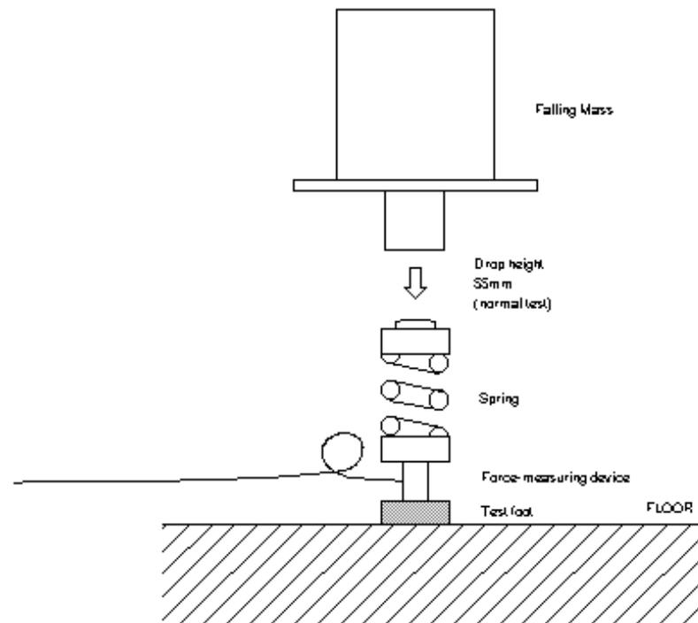
The apparatus consists of the following main components;
