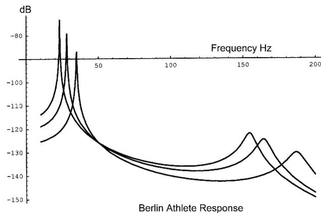
The three curves represent the responses for surfaces with Force Reductions of 50, 40 and 30 % (from left to right). The primary peak below 50 Hz is due to the vibration of the 20 kg mass, and the secondary peak, at 155 to 200 Hz, to the vibration of the 3 kg foot. (It would be 7 % lower in frequency for a 3.5 kg foot)
