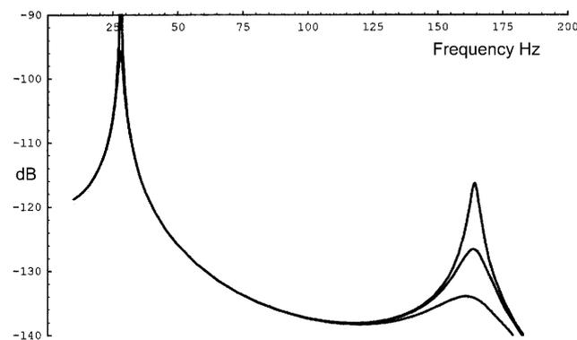
The rationale for a filter with cut-off at 120 Hz appears to be to eliminate the signal from the secondary peak. However, the intensity of the secondary peak is 35 to 50 dB below that of the main peak. So the 120 Hz filter with a reasonably steep cut-off, say 4 pole at 24 dB/Octave, would produce a 6 to 14 dB attenuation at the frequencies of the secondary peak, thus reducing the energy leakage from this peak to about 0.1 to 1
